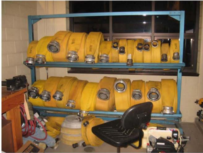
Photograph No. 4 Switching over to rubber fire hoses is the best solution to hose drying energy woes.
