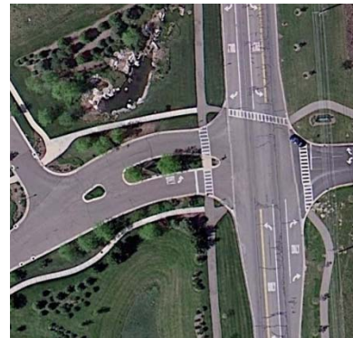
Raised Median at Glenwood Dr Entrance
