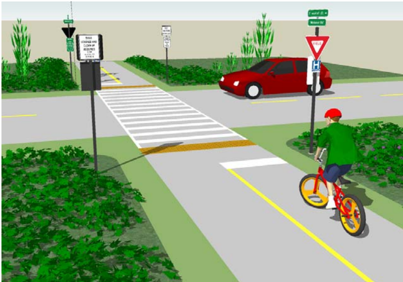
Fig. 5.11C. Trail Signs at Road Intersections Trail View
