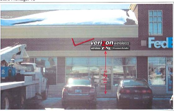
New set of internally illuminated channel letters on raceway Need to cut drywall in interior to access 2' overhang
