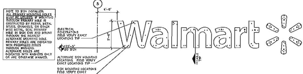
12 SIGN LOCATION 3/4" = 1'-0" 123010 CV022-012a 5'-6" SIGN ON TRILLY BRICK
