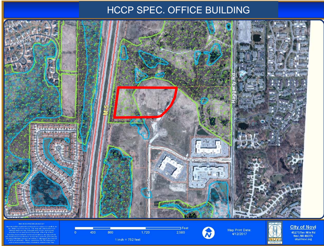
Figure 1. City of Novi Regulated Wetland & Woodland GIS Coverage Map (approximate project boundary shown in red). Regulated Woodland areas are shown in green and regulated Wetland areas are shown in blue.
