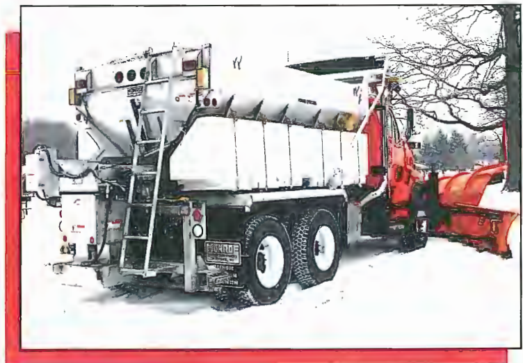
▶ Chassis mount, 14' v-box, 720 gallons of liquid, prewet, custom light package & 3-lane anti-ice corrosion-resistant stainless fenders, top grates, and ladder.
