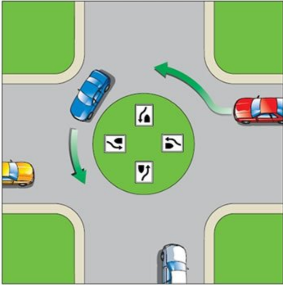
NEIGHBORHOOD TRAFFIC CIRCLE
