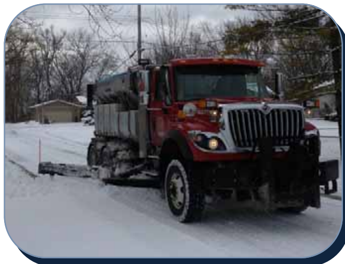
Wing Plows Equipped with Laser Guidance System
