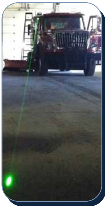
Wing Plows Equipped with Laser Guidance System
