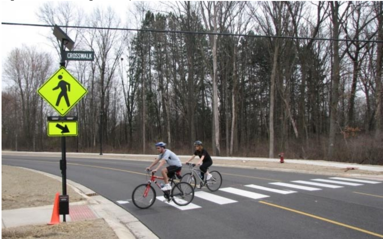
Fig. 5.7H. Rectangular Rapid Flash Beacon
