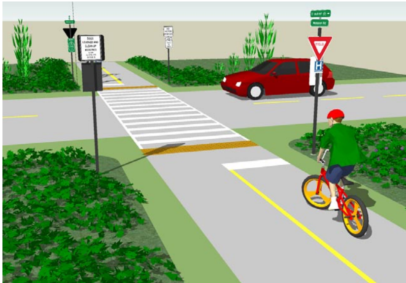
Fig. 5.11C. Trail Signs at Road Intersections Trail View
