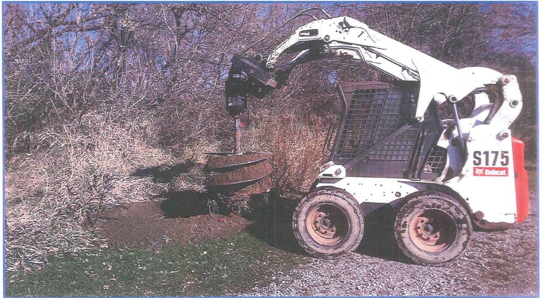
Picture 1: R.C. Tuttle auguring tree planting holes. They will score the sides of the hole with shovels before planting the tree to better able the tree roots to penetrate the hole's walls.
