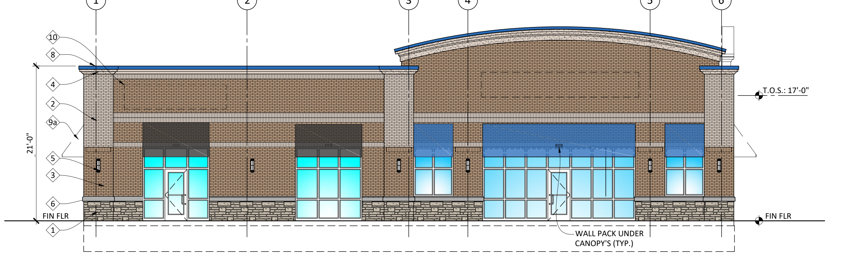
WEST ELEVATION SCALE: 1/8" = 1'-0" AWNING PERCENTAGE: 11%
