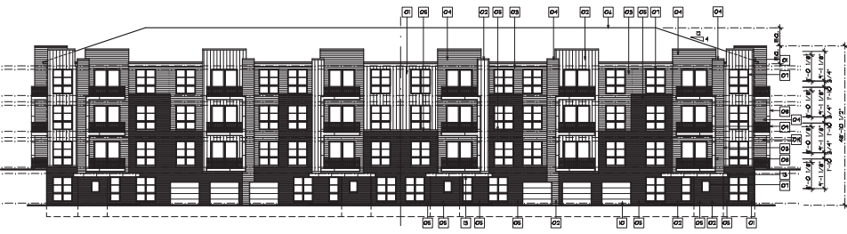
REAR ELEVATION BUILDING 250 BUILDINGS WILL STEP TO FOLLOW FINAL GRADE - SEE CIVIL DRAWINGS SCALE: 1/16" = 1'-0"
