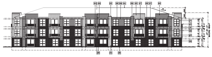
REAR ELEVATION BUILDING 100 SCALE: 1/16" = 1'-0"
