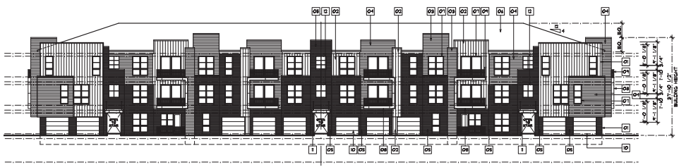
FRONT ELEVATION BUILDING 250 BUILDINGS WILL STEP TO FOLLOW FINAL GRADE - SEE CIVIL DRAWINGS SCALE: 1/16" = 1'-0"
