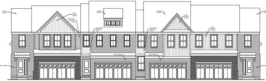
FRONT ELEVATION - HORTON ELITE/DEVONSHIRE Scale 1/8" = 1'-0" FRONT ELEVATION - SANDERS/NEWHAVEN Scale 1/8" = 1'-0" FRONT ELEVATION - HOWE/WETHERBY Scale 1/8" = 1'-0" FRONT ELEVATION - FULMER ELITE/NEWHAVEN Scale 1/8" = 1'-0"
