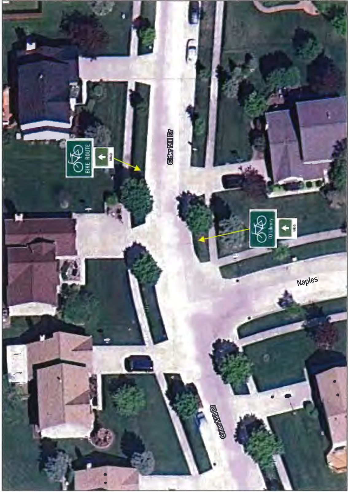
Figure 4a. Confirmatory Signing on Cider Mill at Naples
