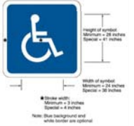
Figure 318-22. International Symbol of Accessibility Parking Space Marking
