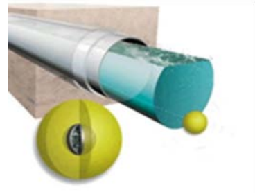
Figure 2: SmartBall Inspection Platform
