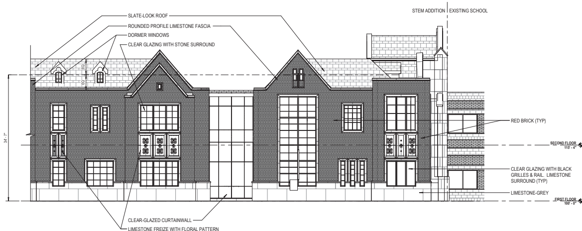
1 PARTIAL NORTH ELEVATION - WEST
