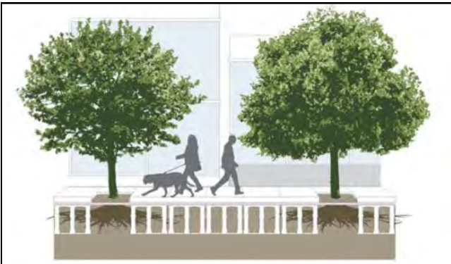
Figure E27: Illustration of silva cells underneath urban trees; source: landscapeperformance.org
